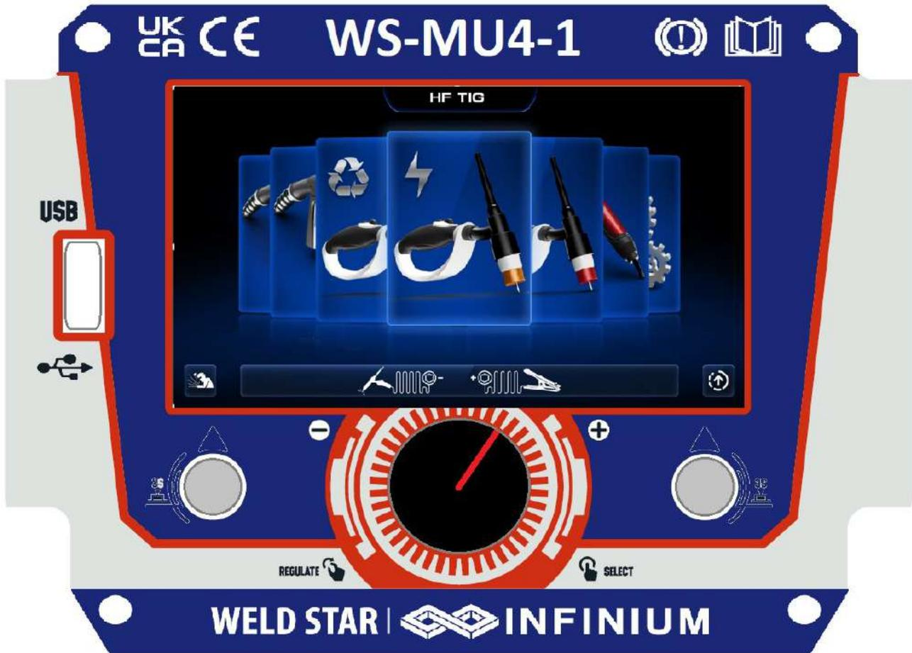
Upon powering ON your MU4-1 and boot up is complete, the control panels main menu will appear on the digital panel as shown above.
