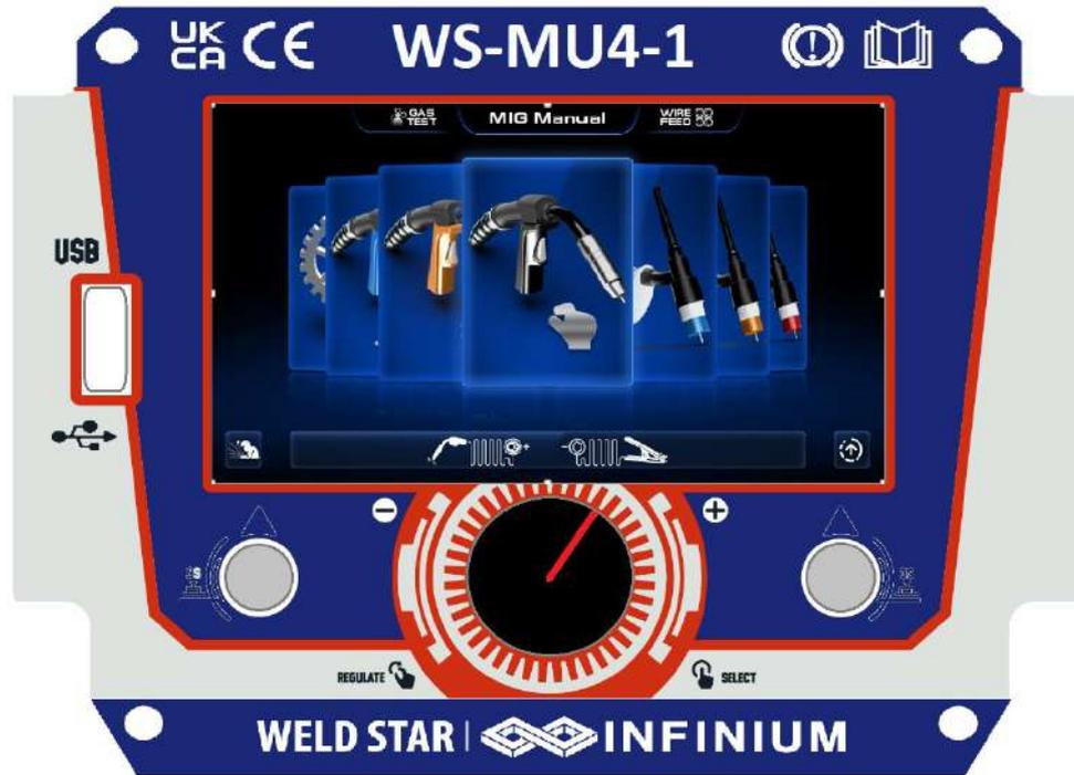
Upon powering ON your WS-MU4-1 and boot up is complete, the control panels main menu will appear on the digital panel as shown above.
