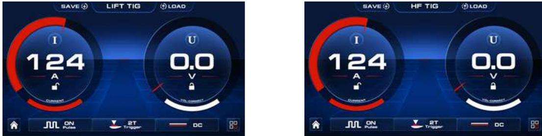
Note that the left circular section offers TIG welding current control and the right section shows TIG voltage, while the bottom row shows Pulse, torch trigger mode and DC/AC output selection. Again, to adjust each setting, simply press the control dial until the parameter you wish to adjust is highlighted in red and then rotate the dial to adjust said parameter, pressing the control dial again stores that parameter setting.
