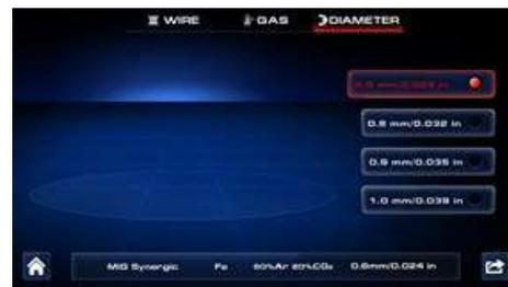
At this point the bar along to bottom of the screen does show the operator welding mode, material, gas and wire size that have selected.
