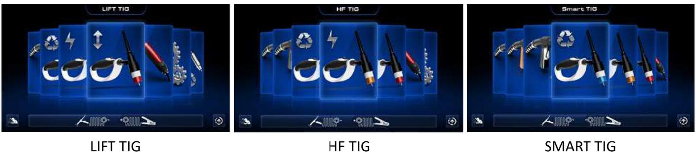
By rotating the main centre control dial you will 'scroll' through the options and by pressing the dial you will enter either Lift TIG, HF TIG or Smart TIG.
