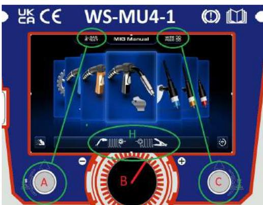
Navigate to one of the MIG welding process options, the example shown left is MIG manual, you will then note that just above the control dial circled 'H' it shows the polarity of the MIG torch and work return lead:
