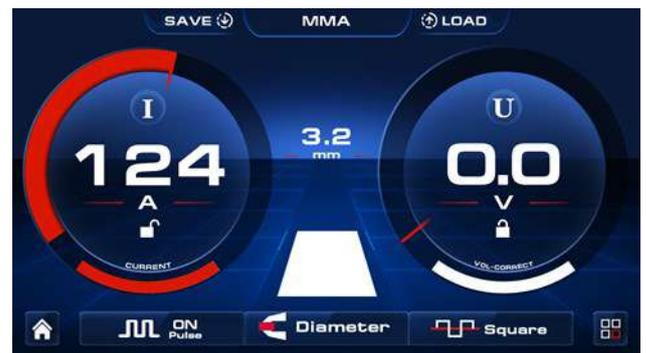
From this screen you can also select and control advanced MMA welding parameters via the icon
