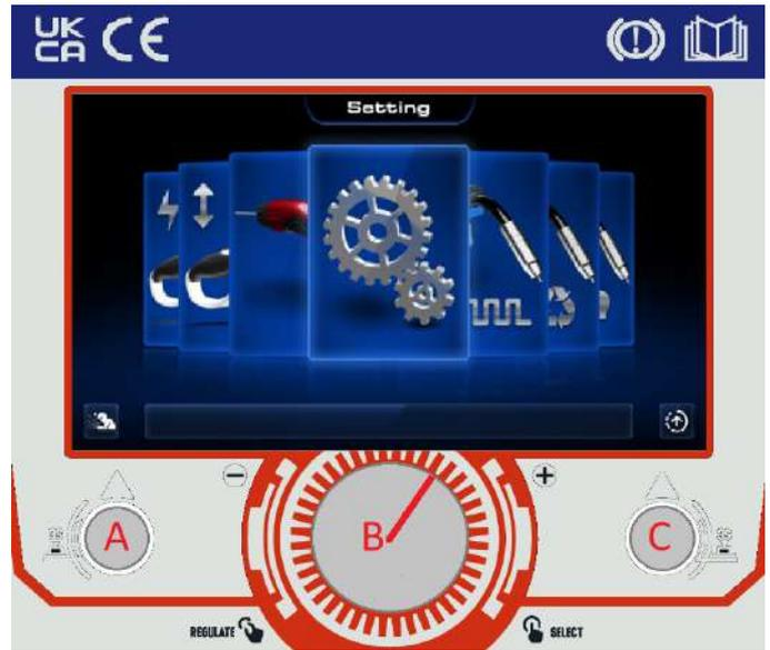
The settings page is divided into two sections 'general' and 'machine' and to switch between these two tabs simply press button 'C' and the tab selected will be highlighted in red.
