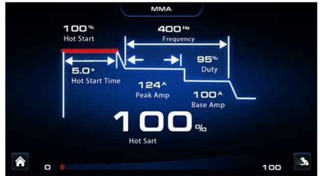
You will note from the image right that the selected parameter being adjusted is Hot Start and you will also note that the bottom bar shows the minimum setting (0) and the maximum setting of (100) % with the variable red bar between going up/down depending where you set the adjustment rotating dial.
