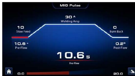
You will note from the above images that the selected parameter being adjusted is Pre-Flow Gas and the bottom bar shows the min setting (0.0) and the max setting of (20) seconds with the lines between going up/down depending where you set the adjustment rotating dial.
