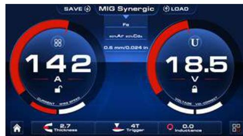
As the above screens show, the left circular section offers either current or wire feed setting and the right section shows voltage/arc length and these options can vary depending on which MIG process has been selected.
