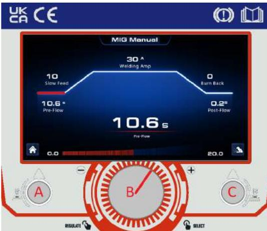
Following on from the instructions on the previous page, if you press and release (short press) button 'C' you will now enter a new screen (shown left) that allows the operator to select and adjust more advanced (in this case) MIG settings such as:
